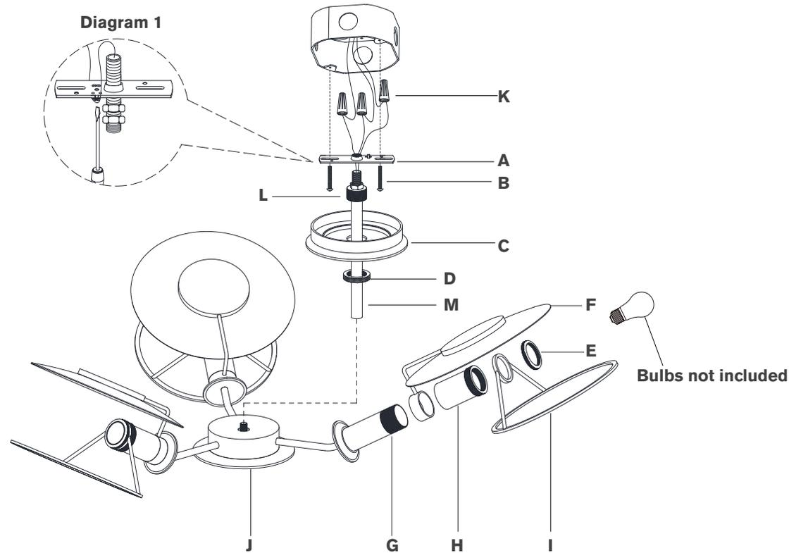
11. Install canopy (C) to mounting plate (A) and secure with collar ring (D).
