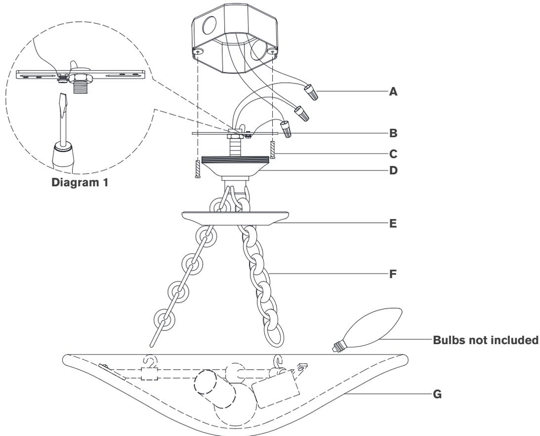
11. Connect fixture neutral wire (ribbed) to the supply neutral wire (usually white) using wire nut **(A)**.
